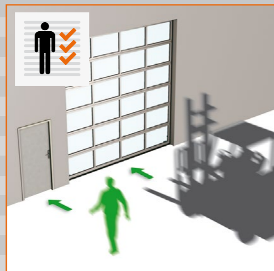
Completely separate doors for pedestrians and goods.
